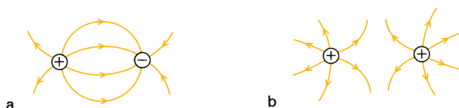
Figure 2.23 Electric fields around a pair of opposite charges, and a pair of charges with the same sign.
